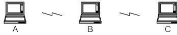
Fig. 1. A multi-hop network for observing PDRT where the multicast tree is constructed in A-B-C.
